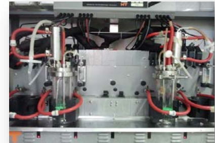
Set up of a Large-scale biofilm cultivation of P. haloplanktis TAC125
